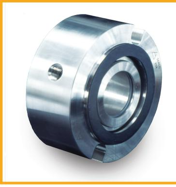
The SEPCO® VSR is a single, external, cartridge-mounted, rotary seal designed for installations where shaft deflection exceeds the limits allowed by off-the-shelf cartridge seals. Excessive radial clearances designed in the seal make it ideal for vertical turbine pumps in power plants, pulp & paper mills, municipalities, and applications in relatively clean, lubricating fluids.
