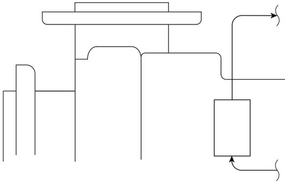
Install pressure gauge in lantern ring inlet connection to determine actual stuffing box pressure. Maintain flush pressure at 15-20 psig over stuffing box pressure.
