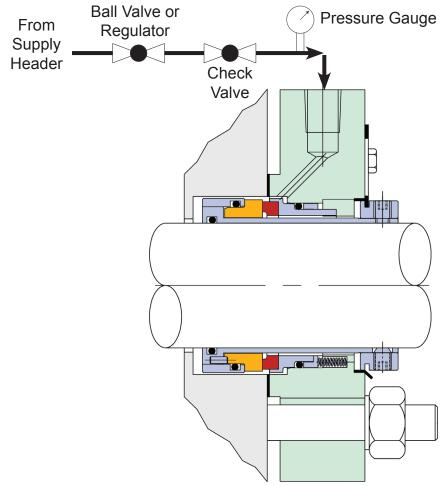
Note: Install restriction bushing or lip seal in bottom of stuffing box prior to installing seal
