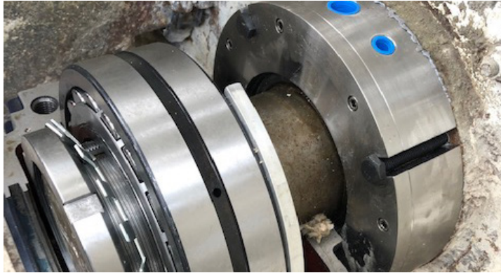
SEPCO SAS installed for a cement mixer
